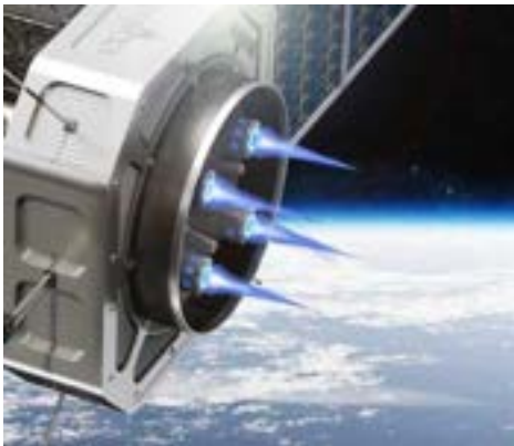
Electric Propulsion (Ion Thruster)
